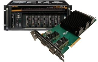
Alternatively, Chimera can be installed as a test module (2-slots) in a ValkyrieBay chassis. The impairment functionality then becomes available via ValkyrieManager
