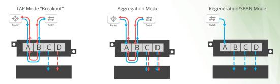
Port-to-Port Aggregator with Port Mapping Filtering
