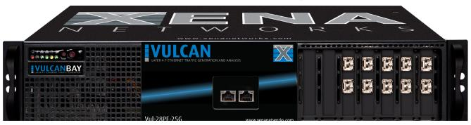
VulcanBay is a scalable Gigabit TCP test chassis that offers extreme performance for stateful traffic load testing, analysis and characterizing of Ethernet equipment and network infrastructure. It supports 1/2.5/5/10/25/40GE interfaces and can be used for simulating millions of real-world end-user environments to test and validate infrastructure, a single device, or an entire system.
